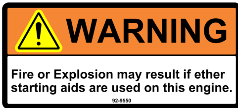
Figure 2. Do Not Use Ether Starting Aids (Near Engine)
